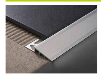
The 20° slope of the anodized aluminum RAMPTEC ZRR profile provides a safe and progressive transition between two different floor levels. The vertical edge has a dovetailed internal cavity that maximizes grout and adhesive grip on load bearing points.
